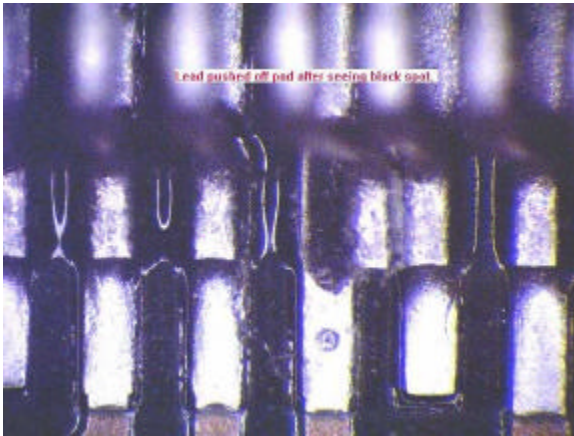
Figure 3 – QFP with Cracked and Shifted Lead
