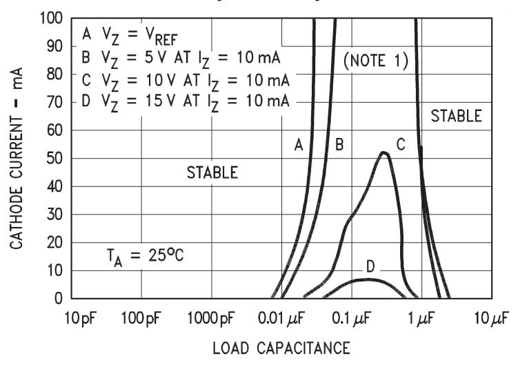
Note 1: The areas under the curves represent conditions that may cause the device to oscillate.
