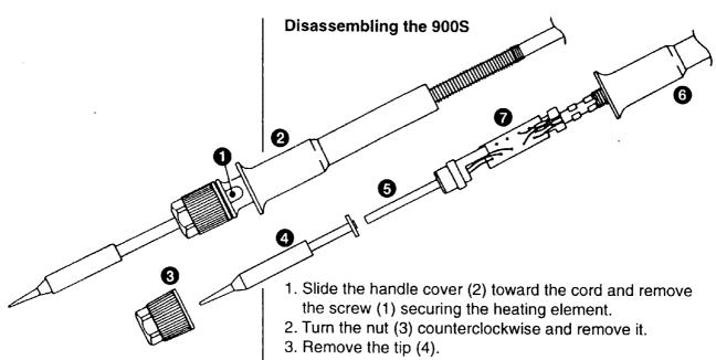
4. Pull both the heating element (5) and the cord toward the tip of the iron and out of the handle (6).
