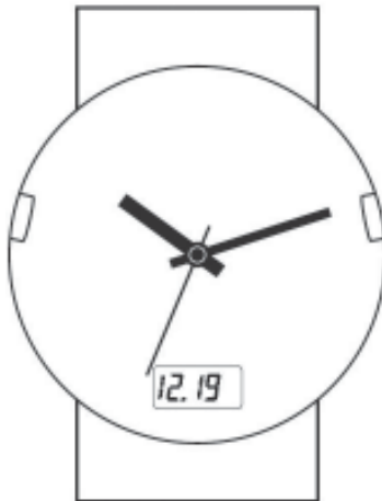
Figure 2. Analog clock display with digital inset for date information.
