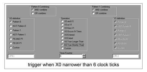
In this case we calculate the counter/timer value by dividing the clock speed. For instance, 60ns with a 100MHz (10ns) clock, gives a counter value of 6.
