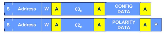
No need to access Configuration and Polarity registers once programmed
