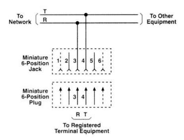
**RJ-17C:** Provides a single-line bridged connection of tip and ring to special telephone sets or ancillary equipment (e.g., ECG machines) in hospital critical-care areas. Only registered equipment conforming to Article 517 of the 1978 National Electrical Code is permitted to connect to this jack arrangement. This jack differs from the RJ-11C in that tip and ring appear on pins 1 & 6 rather than 3 & 4.
