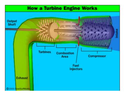
In this engine, air is sucked in from the right by the compressor. The compressor is basically a cone-shaped cylinder with small fan blades attached in rows (eight rows of blades are represented here). Assuming the light blue represents air at normal air pressure, then as the air is forced through the compression stage its pressure rises significantly. In some engines, the pressure of the air can rise by a factor of 30. The high-pressure air produced by the compressor is shown in dark blue.
