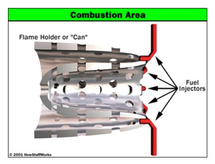
The **injectors** are at the right. Compressed air enters through the perforations. Exhaust gases exit at the left. You can see in the previous figure that a **second set of cylinders** wraps around the inside and the outside of this perforated can, guiding the compressed intake air into the perforations.
