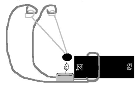
The candle flame will heat up the magnetic material until it loses its ability to be magnetized. Gravity will then pull it away from the magnet (and thus away from the flame). The magnetic material will cool down a little bit once it is away from the flame, and regain its ability to stick to the magnet. The magnet will then pull it up into the flame, and the whole process
