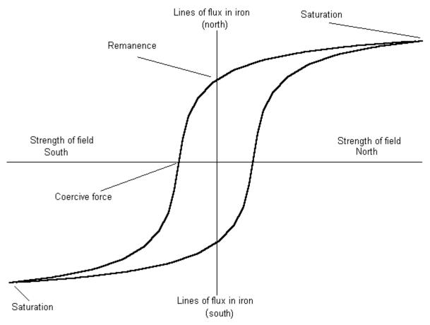
We call the magnetic flux density that remains in the iron when we remove the external field the remanence. We call the strength of the external field needed to demagnetize the iron the coercive force.
