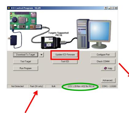
After reflashing the generic (PIC16, v1.29) hex file into a sick ICD using a good ICD, connect the recovered ICD to the serial port and target (For this the target processor and the ICD does not need to match, you're just getting power from the target!) and use ICD.EXE to update the current FW version for PIC16 or PIC18 to match the target processor.
