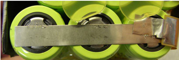
Insufficient welds that are not fully on the tabs
