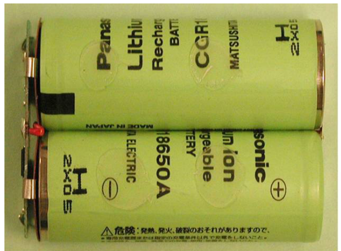
No insulation was used between these cells
