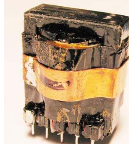
Replace the gauss field shield around the transformer tightly and solder together being careful to not melt through the tape underneath.
