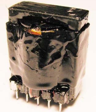
Apply varnish or other coating to glue the assembly together. Extra varnish in the center leg space will help keep the cores held tightly together.
