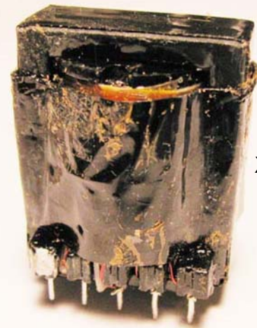
Wrap the shield to core insulator tape around the transformer.
