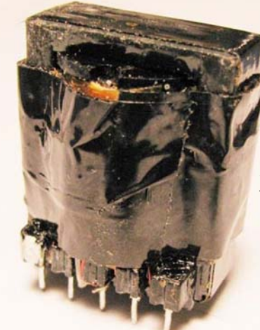
Wrap the transformer with the outer insulation tape.
