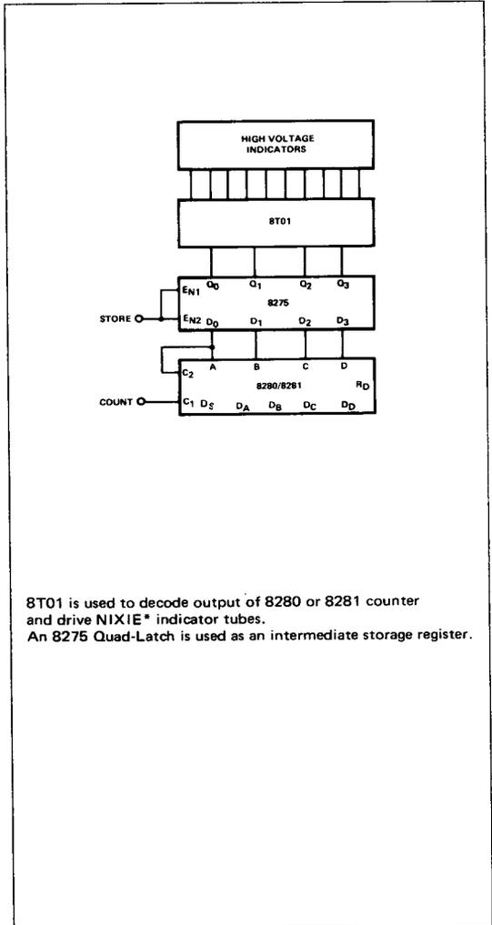
8T01 is used to decode output of 8280 or 8281 counter and drive NIXIE® indicator tubes. An 8275 Quad-Latch is used as an intermediate storage register.
