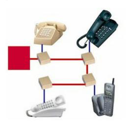
Residential wiring is most often installed in a "loop-through" configuration, where wire goes from the phone company's entry point to one room, then another, and another, and another, in a string. The phone jacks are wired electrically in parallel, but physically in series, and a break in the series can knock out phone service in several rooms 'after' the break.
