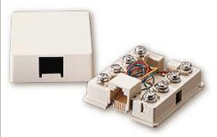
The **surface jack**, is a cube, roughly 2 inches by two inches by 3/4 of an inch, and mounts on the surface of the wall. It is usually installed after a wall is constructed, often with wire stapled to the **baseboard**. They are available in a variety of colors, with connections for two, three or four pairs.
