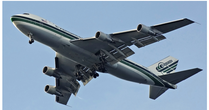
Fig 7. This Evergreen B747 has its flaps fully extended for landing and it is clear that the size of the wing has been considerably increased.
