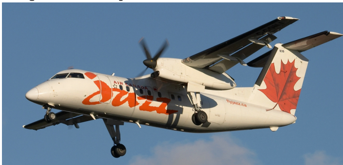
Fig 13. The high wing configuration used on the Dash-8 keeps the propellers clear of the ground, and eliminates the need for air-stairs, but look how long the main undercarriage has to be.
