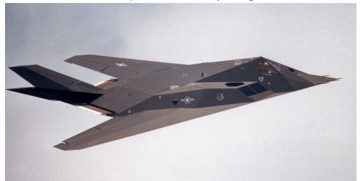
Fig 11. The F-117 Nighthawk is so inherently unstable that it would be uncontrollable without a computer assisted stabilization system.
