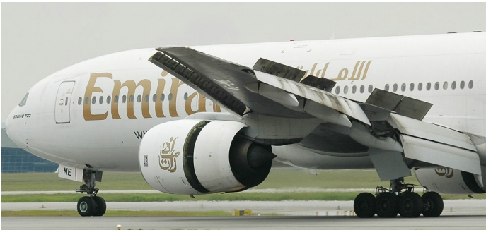
Fig 6. An Emirates B777 after touchdown with spoilers raised and reverse thrust engaged. It can be seen how much the leading and trailing edge flaps have altered the curvature of the wing.
