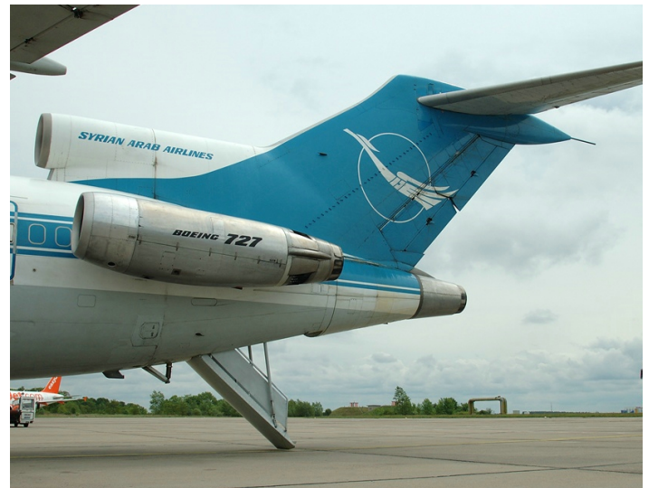
Fig 14. The horizontal stabilizer of the B-727 had to be mounted on top of the fin in order to be clear of the rear-fuselage mounted engines. Note that the entire surface is moveable to be able to provide the required degree of control effectiveness. A big advantage of mounting the engines so close to the centre-line is the improvement in handling quality in the event of an engine failure.
