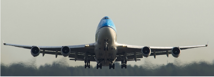
Fig12. Most airliners use a low wing configuration. This shortens the landing gear, and keeps the wings and engines lower to the ground for ease of maintenance and refuelling. They rely on the dihedral (upward bend) of the wings for stability.
