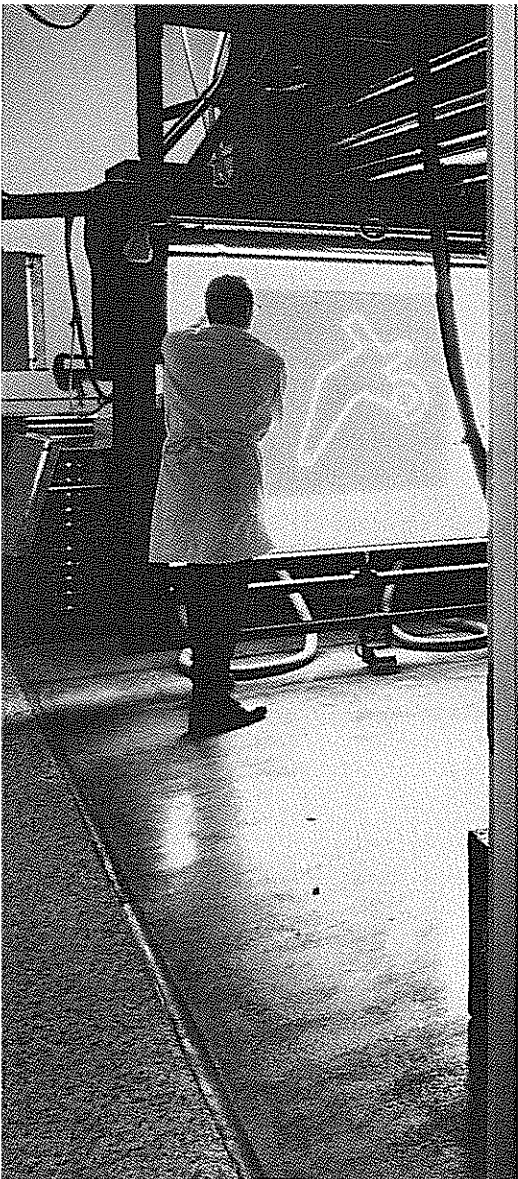
FIGURE 10: The artwork is placed on the backlit copyboard and the precision camera carefully focused.
