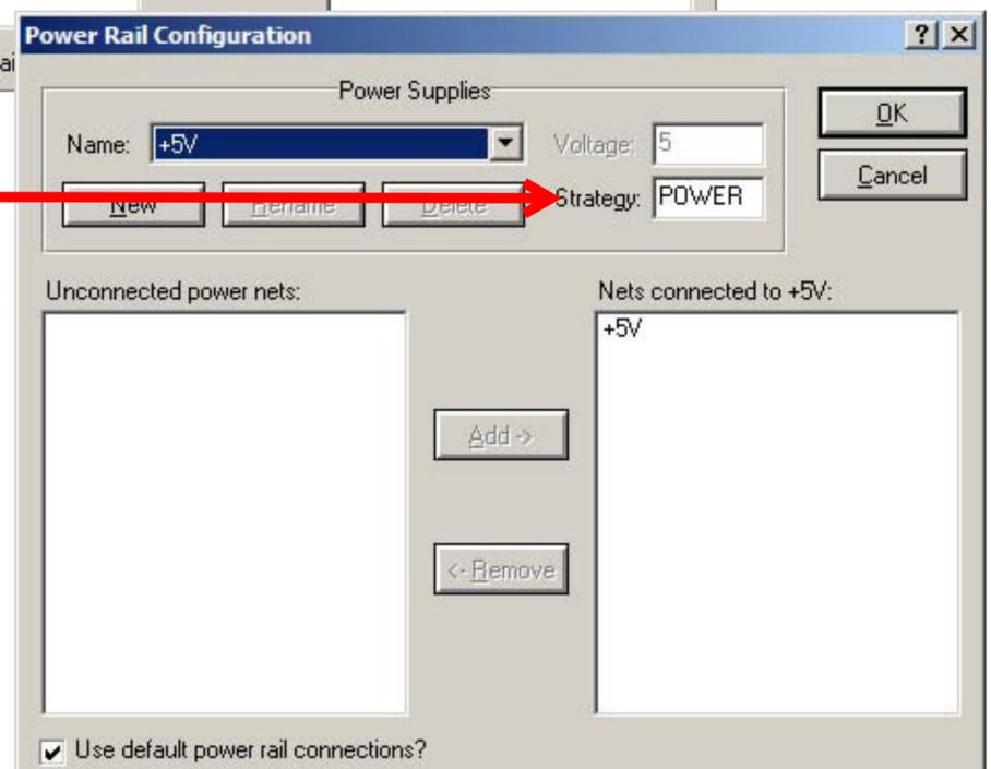
From this point on, ANY terminal with the name "+5V" will be connected to this power rail. In ARES, power and signal nets may be displayed with different colors and treated with different routing rules (Strategies).
